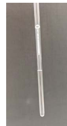
Glass capillary within NMR tube
